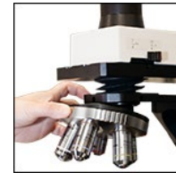
Click to Enlarge The objectives can be changed by manually rotating the front face of the nosepiece.
